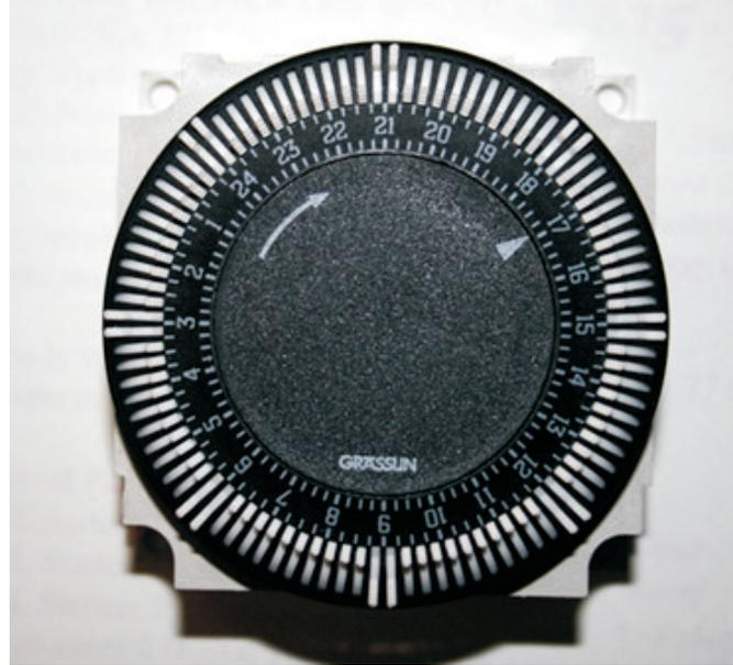
In this picture there are 8 Defrosts per 24hrs of Refrig Run. Two Pegs are pulled out (30 mins) at 24, 3, 6, 9, 12, 15, 18, 21. This is a total of 4hrs of Defrost in 24hrs.
