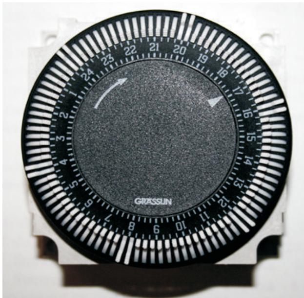
In this picture there are 6 Defrosts per 24hr of Refrig Run . Two Pegs are pulled out (30 mins) at 24, 4, 8, 12, 16. This is a total of 3 hrs of Defrost in 24hrs.
