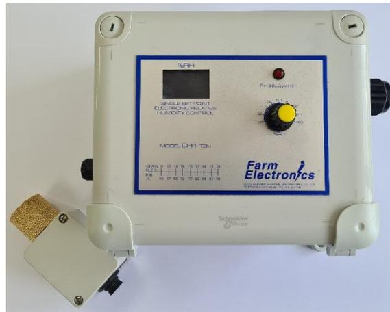
The controller utilises a single control set point adjustable from 20 - 90% RH. When the humidity drops below the pre-set level the internal control relay energises as indicated by the Red LED above the set dial. The controller has inbuilt time delays on the control relay to prevent Hunting of electrical motors etc.
